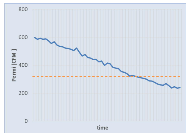
Figure 2: Defining critical limit (orange line) based on PERMI results
