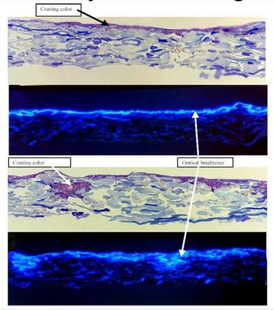
Dense sheet – small penetration of coating color and good coating coverage and gloss.
