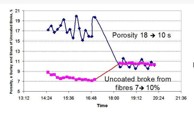
Very small changes in the broke levels can have a big effect on paper porosity (increasing or decreasing). In this case addition of uncoated broke has increased porosity.
