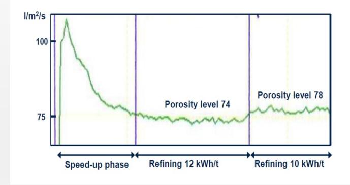
A very small change in refining control can be clearly seen in the porosity measurement. The units of porosity numbers are I/m2/s.
